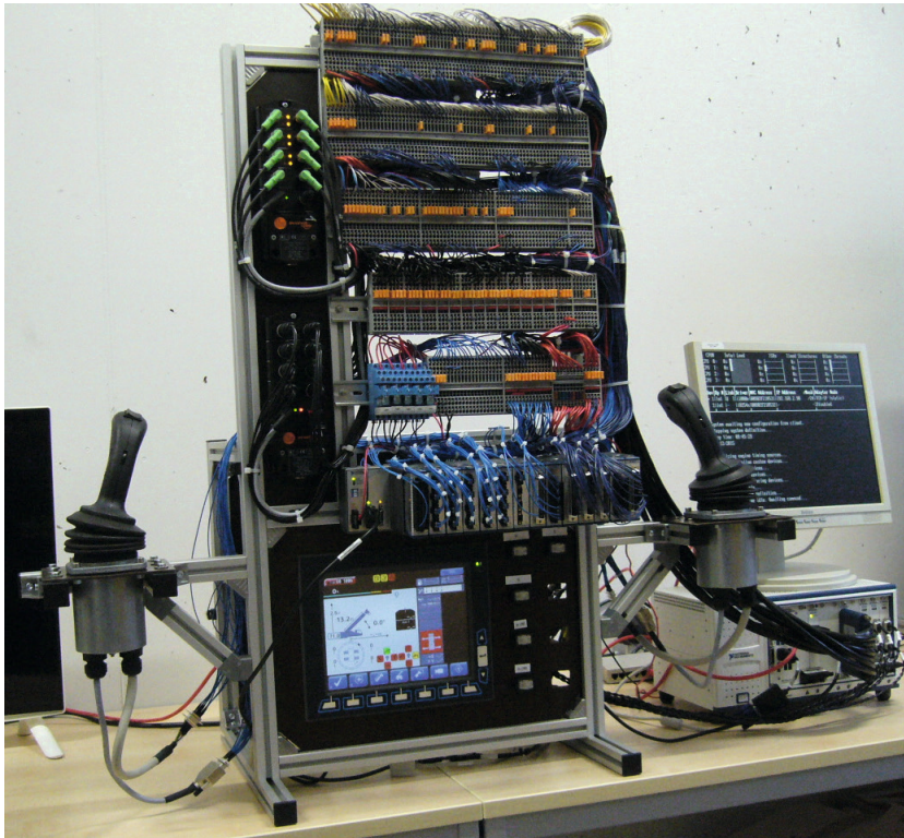
Figure 2: Hardware-in-the-Loop Teststand for a Mobile Machine
